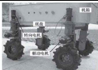
图1-14 全方位转动农业机器人 Fig.1-14 Rotate agricultural robots in all directions
